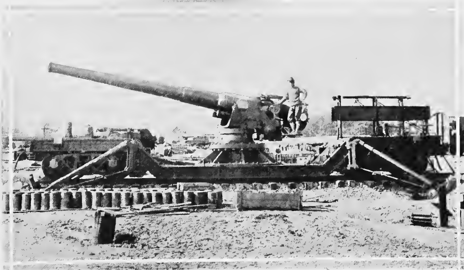
7-Inch, 45-Calibre Navy Gun, Barrette Carriage, Mounted on Railway Car, Model 1918 MI
